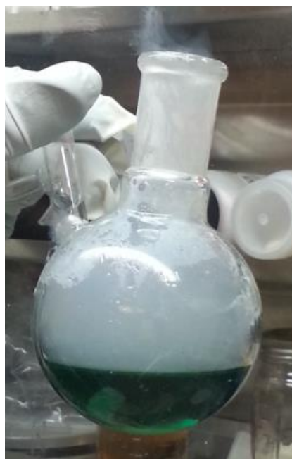
Figure 6. Photograph of basic \text{NiCl}_2 -EMIM- \text{AlCl}_3 solution.
