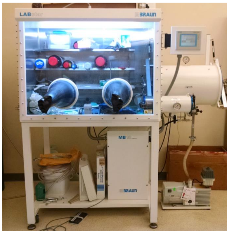
Figure 1. Photograph of MBRAUN LABstar glove box workstation.
